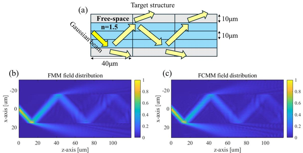
Fig. 1. FCMM simulation of simple waveguide for tilted gaussian beam. The structure was divided into five local regions along the x-axis, each with a width of  $10\mu\text{m}$ , and consisted of three layers, with a thickness of  $40\mu\text{m}$ , along the optical axis. (a) Structure schematic. (b) Field visualization results (FMM). (c) Field visualization results (FCMM).
